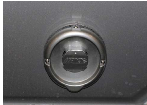
Vent for Alde unit on driver's side exterior
