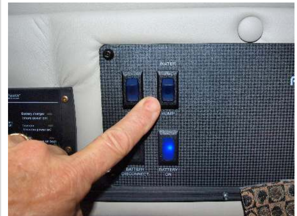
Water pump switch with 2500 watt inverter
