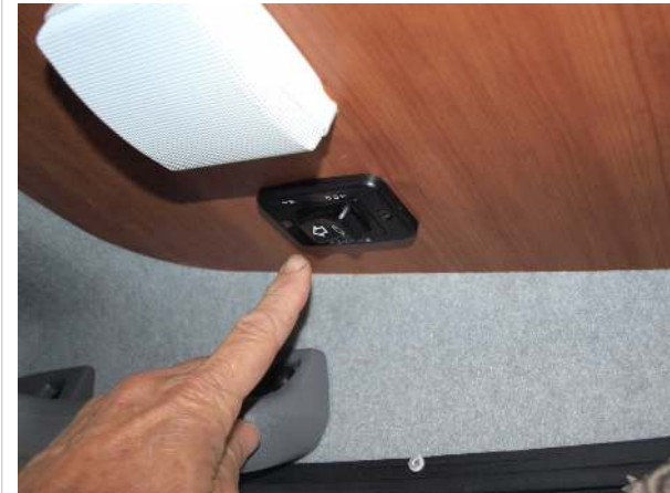
Awning switch above front passenger seat
