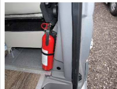
Fire extinguisher located behind front passenger seat
