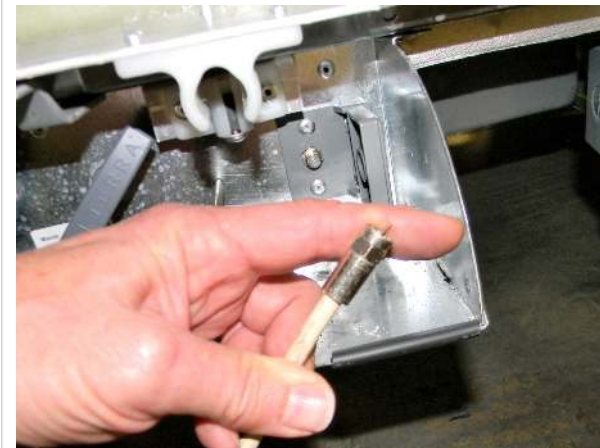
Coaxial TV connecting wire with screw-on end
