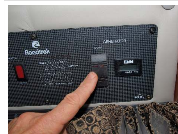
Generator switch and hour meter (optional)
