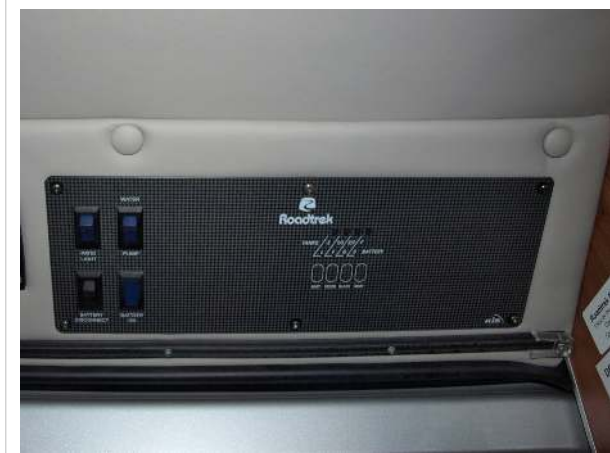
Monitor Panel for CS with optional 2500 watt inverter and engine generator
