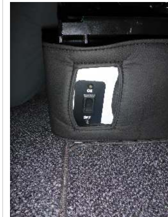
The switch is located on the inboard side of the passenger seat pedestal
