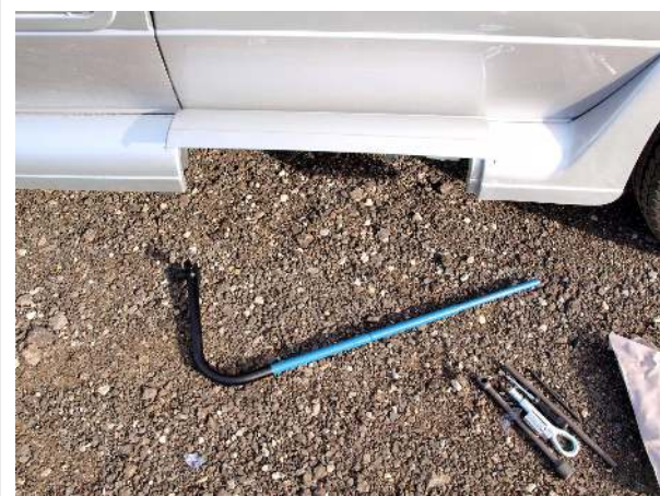
Assembled lever to lower spare tire carrier
