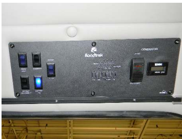
Monitor Panel with 1250 watt inverter and optional propane generator
