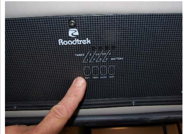
Tank and battery level indicators
