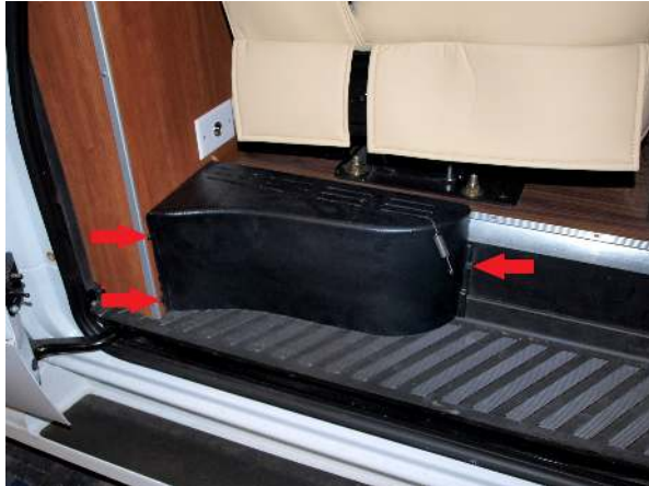
City water valve access - loosen the screws (locations indicated by red arrows) and remove the radiator cover
