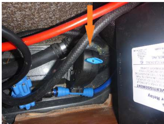
Alde frost protection normal position - blue handle is pointing parallel to the water line, blue button at base (see arrow) is in
