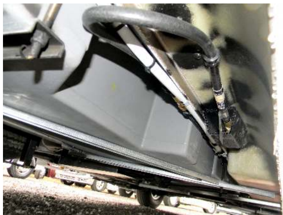
High pressure BBQ pigtail, in stowed position in front of passenger rear tire
