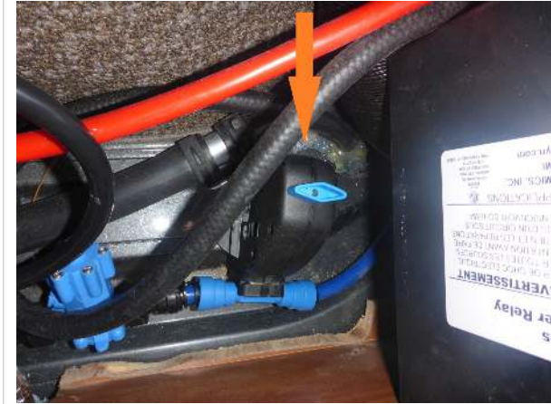
Frost protection valve in normal operating position
