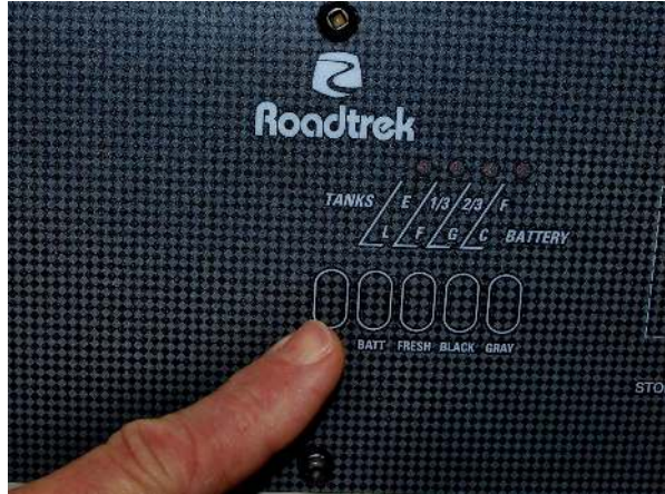
Tank level and battery charge indicators
