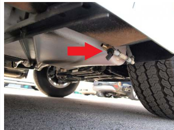
Freshwater tank drain valve
