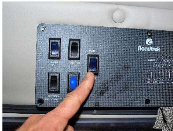
Water pump switch with standard inverter
