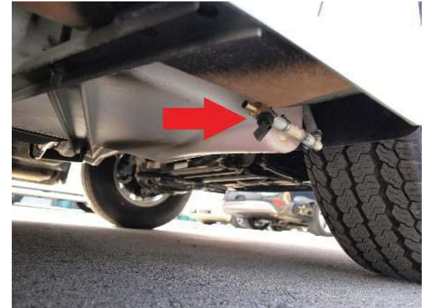
Freshwater tank drain valve
