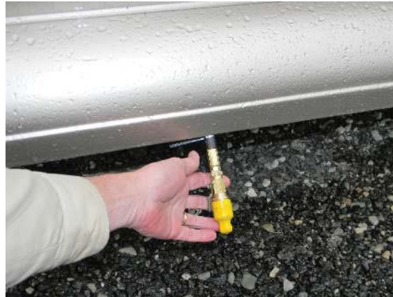
Propane pigtail, removed from retaining enclosure
