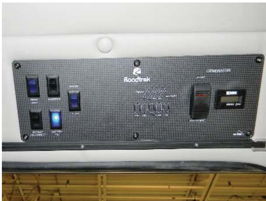
Monitor Panel with 1250 watt inverter and optional propane generator
