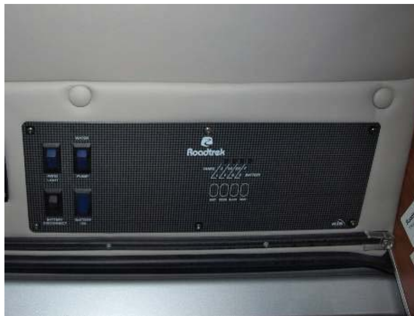
Monitor Panel for CS with optional 2500 watt inverter and engine generator
