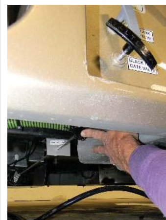
Chevy macerator manual crank knob
