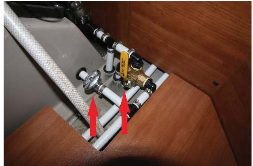
Tank selector lever in the interior (vertical) position
