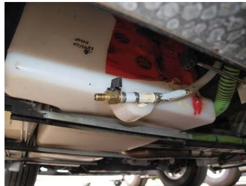
Freshwater tank drain valve, shown closed
