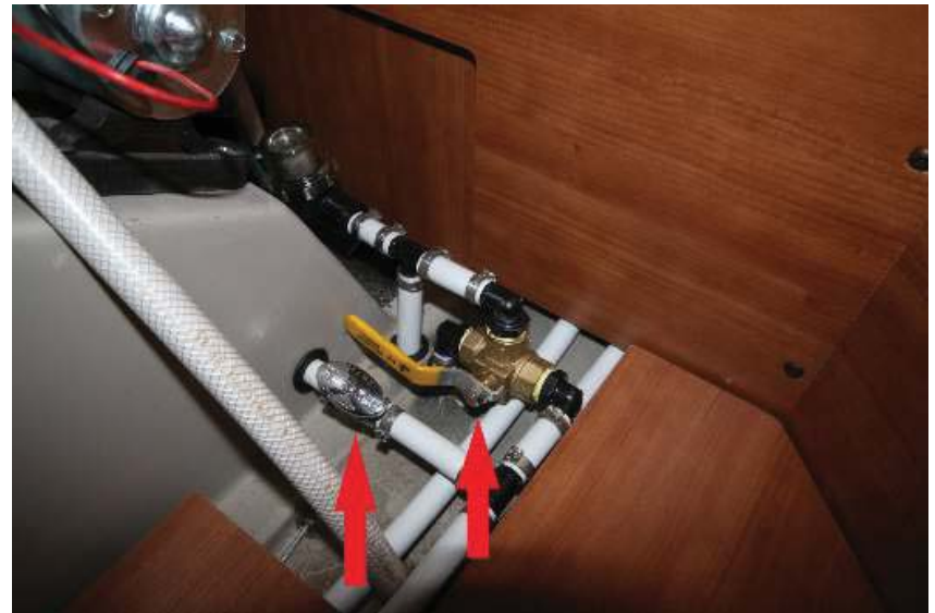
Tank selector lever in the exterior (horizontal) position
