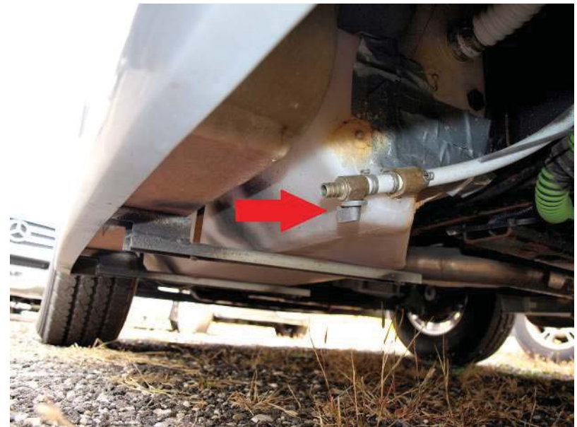
Freshwater tank drain valve
