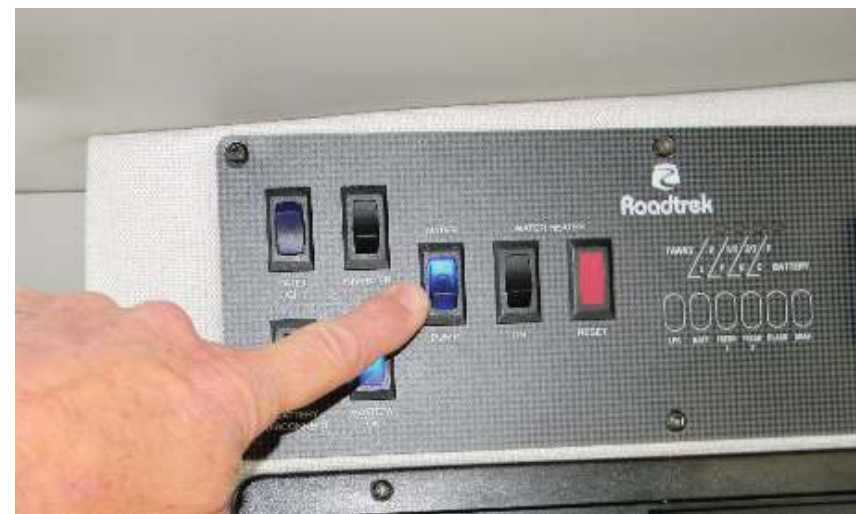
Water pump switch on (blue indicator light lit)
