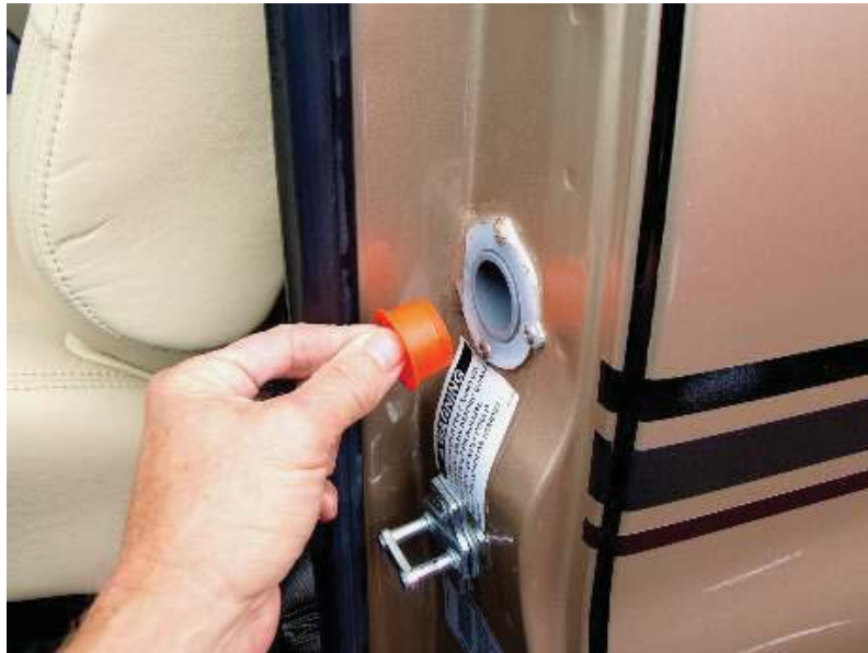
Front (exterior) tank gravity fill
