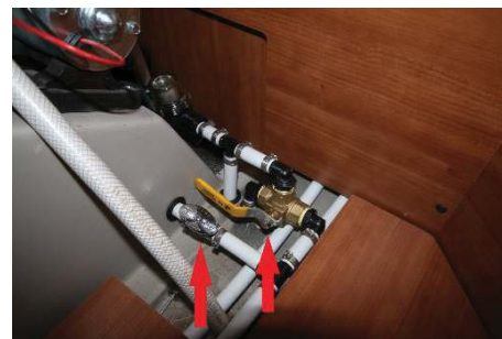
Tank selector valve in exterior tank position (colored plastic handle pointed toward driver's side of Roadtrek). Tank isolator valve is open, allowing water to drain from interior tank to exterior tank.
