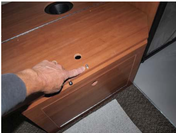
Screw to open water valve enclosure
