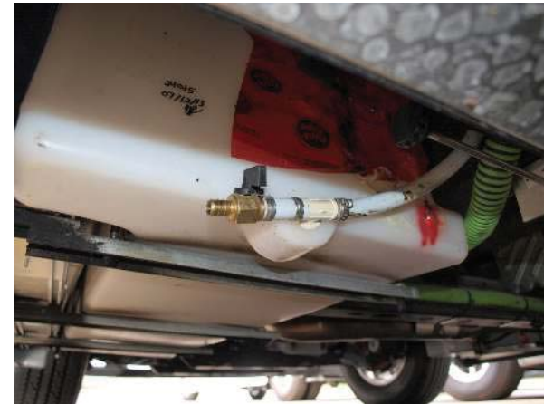
Exterior tank drain, under driver's door step
