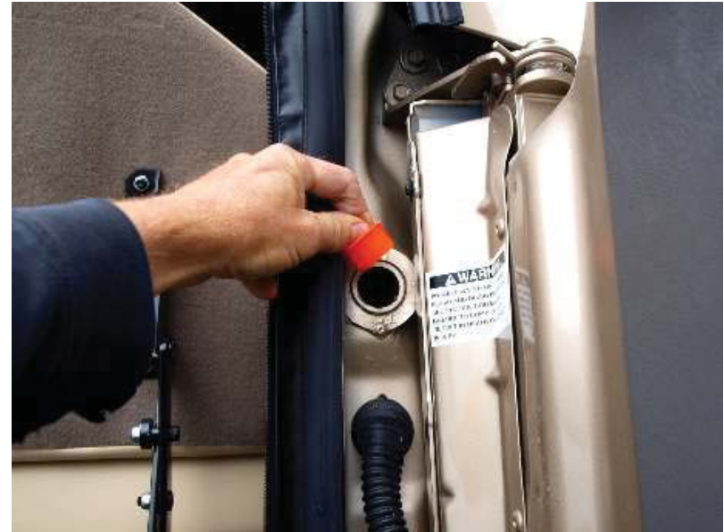
Rear (internal) tank gravity fill
