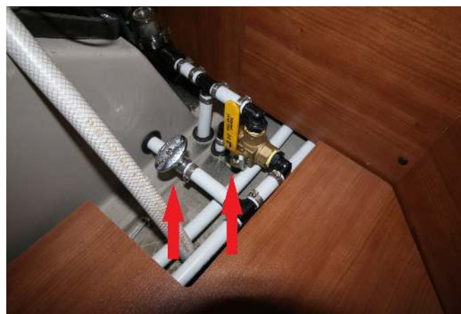
Tank selector valve in interior tank position, with the colored plastic handle pointed up. Tank isolator valve is closed, preventing water from flowing into the exterior tank.
