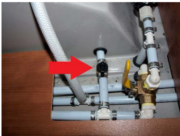
Tank isolator valve in open position (black plastic handle pointed along line). This valve is located inside the water control enclosure under the driver's side bench to the left of the refrigerator.
