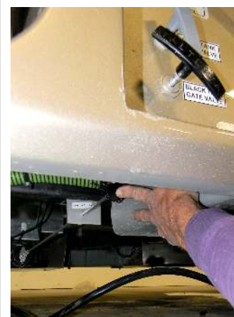
Chevy macerator manual crank knob
