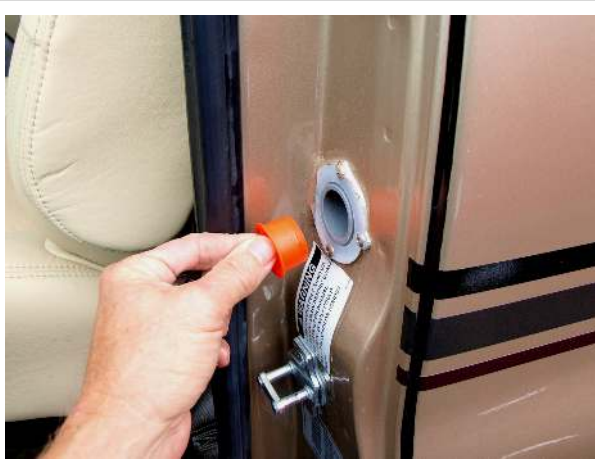
Front (exterior) tank gravity fill
