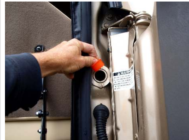
Rear (internal) tank gravity fill
