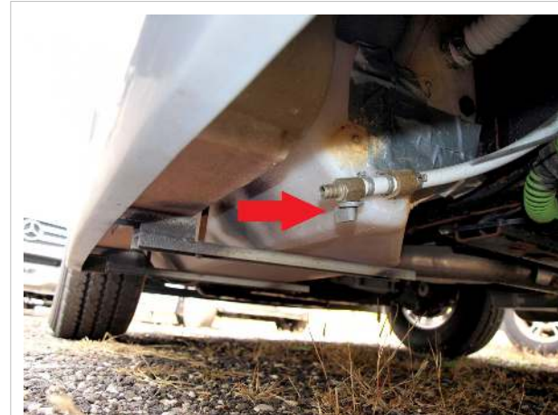
Fresh water tank drain, under driver's doorstep
