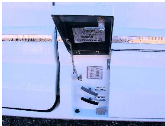
Driver's side front access door showing tank dump valves
