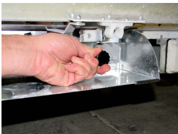
Sprinter macerator manual crank knob
