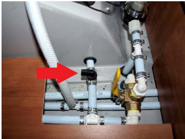
Tank isolator valve in closed position (black plastic handle pointed toward the back of the vehicle). This valve is located inside the enclosure, under the driver's side bench.
