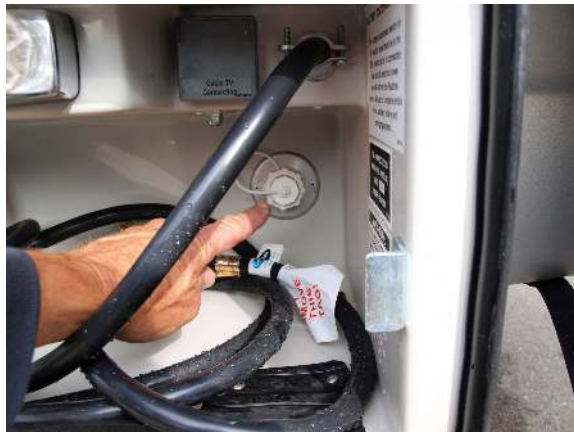
City water fill location
