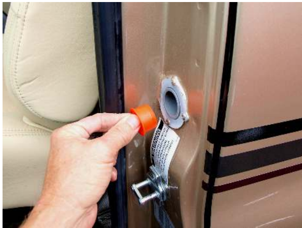
Exterior tank fill location (driver door pillar)
