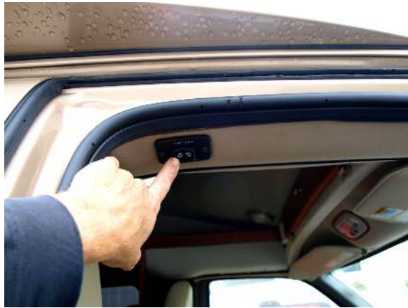
Awning power switch
