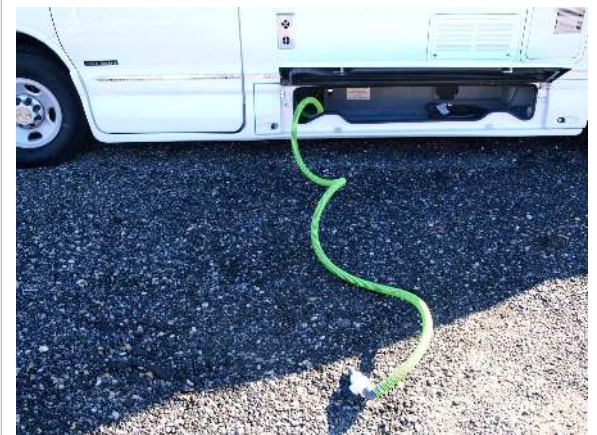
Driver's side center access door houses power cord and waste hose
