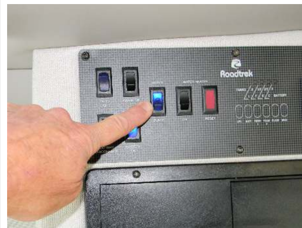
Water pump switch on (blue indicator light lit)
