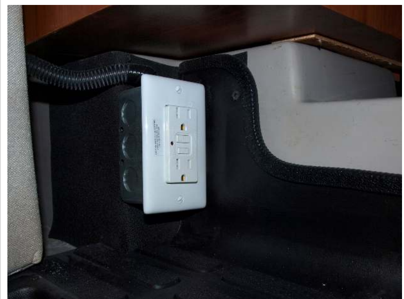
GFCI outlet under rear passenger side seat
