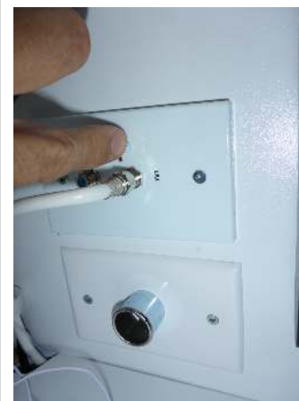
Push the small button to select Antenna or Cable
