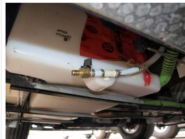
Exterior tank drain, under driver's door step
