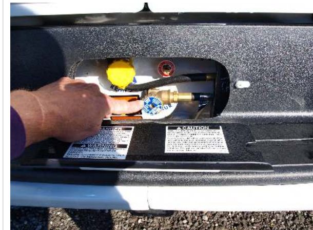
Propane tank main shutoff - fill valve capped with yellow cap
