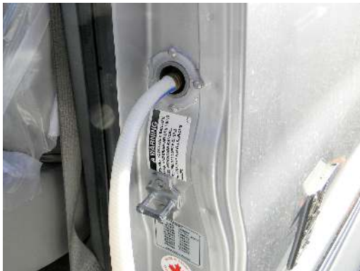
Filling the exterior tank
