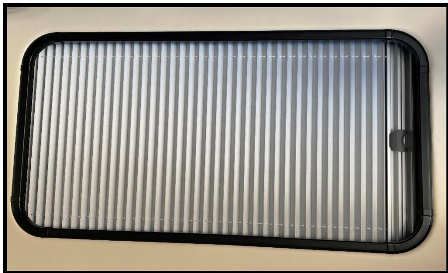
18.1 The side window screens – nightshade side
