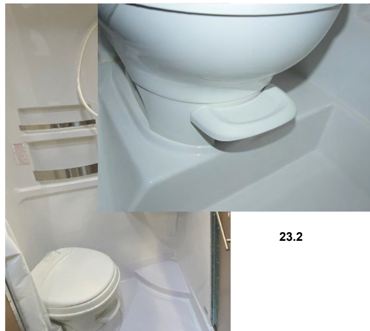
TP holder Not a handle – will not support weight
