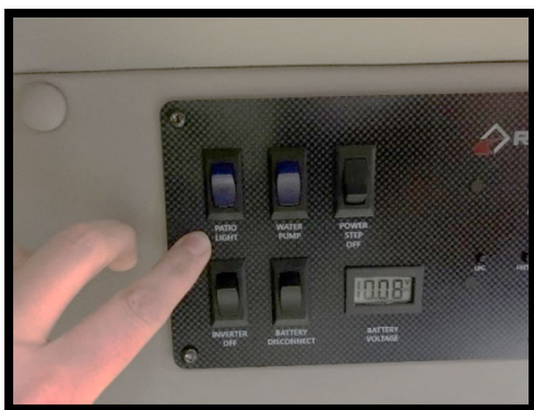
44.1 Patio Light Switch
