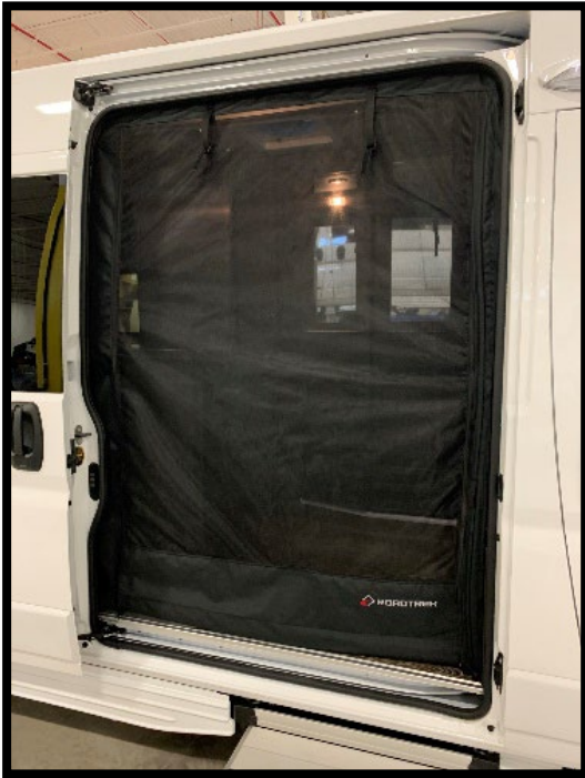
Side screen closed with bug net
