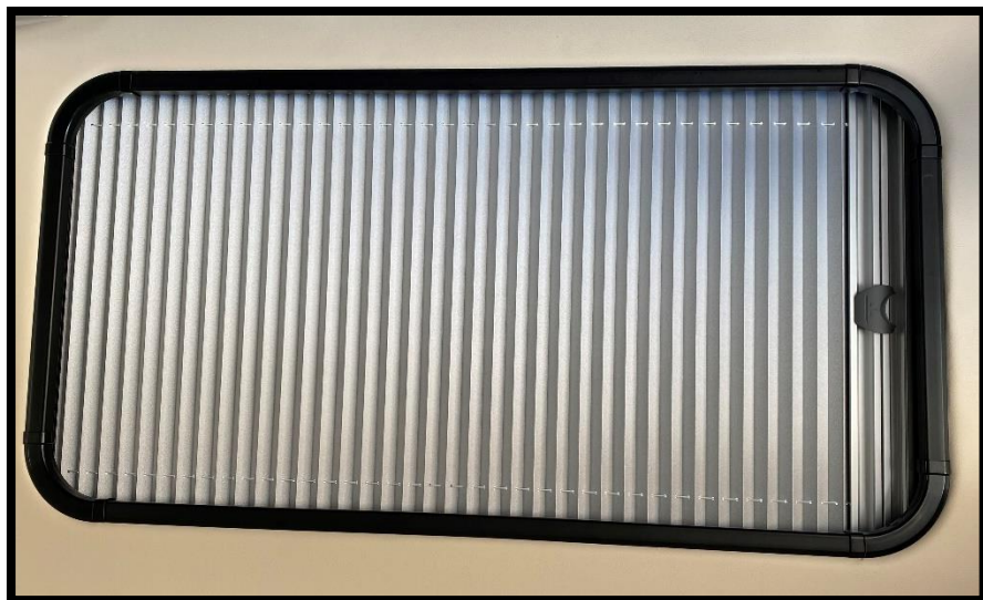
18.1 The side window screens – nightshade side
