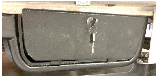
34.5 Locking storage compartment for flexible macerator hose
