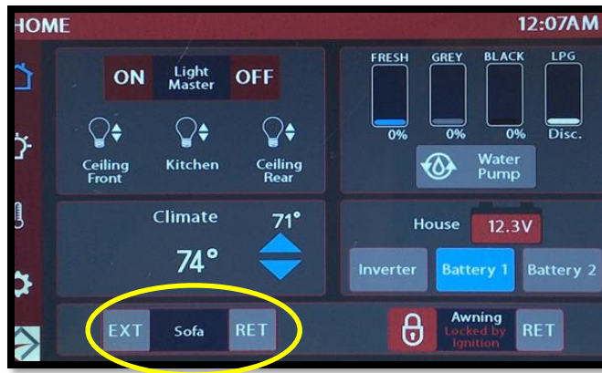
22.2 Sofa controls on monitor panel
