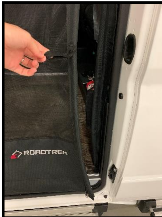
Side screen showing magnetic close
