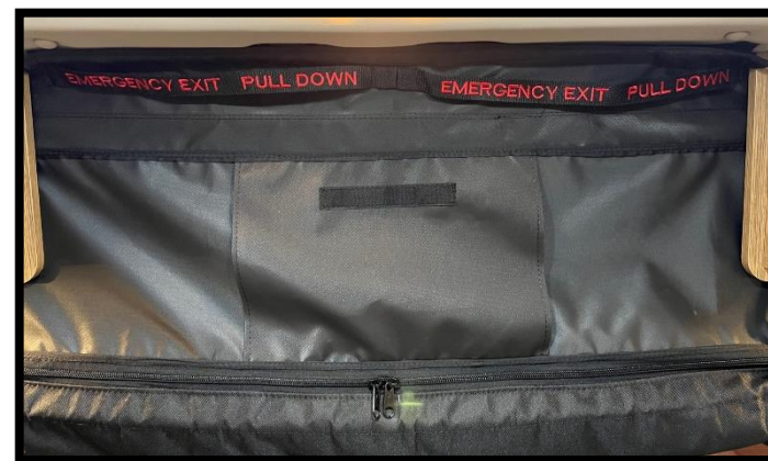
Screens are attached by heavy duty Velcro. Pull on both straps to detach screen in an emergency.
