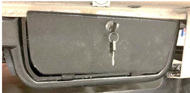
34.5 Locking storage compartment for flexible macerator hose
