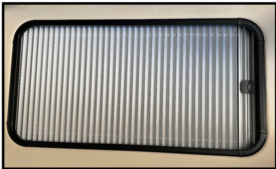
18.1 The side window screens – nightshade side
