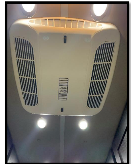
35.3 Roof-mount air conditioner
