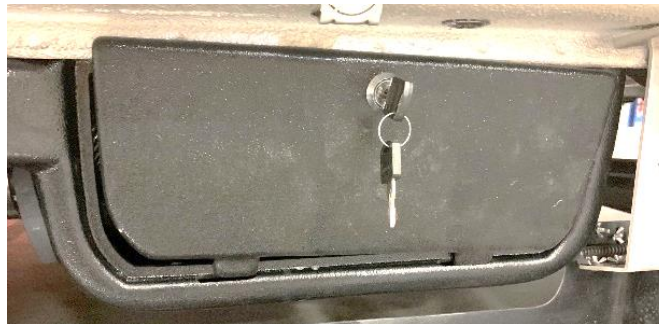
34.5 Locking storage compartment for flexible macerator hose
