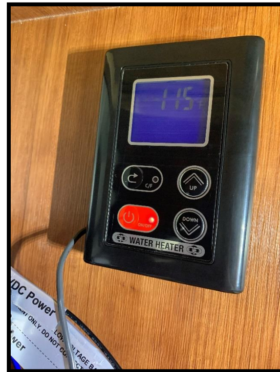
28.3 Water heater control panel
