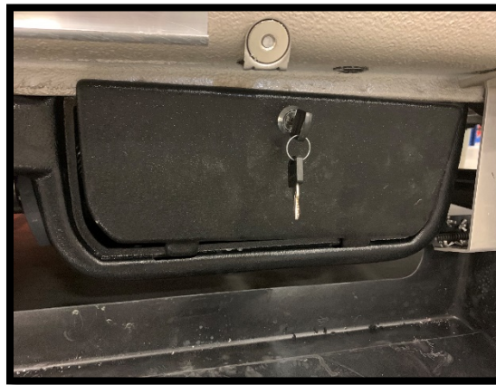
Picture 35.5 Locking storage compartment for flexible macerator hose
