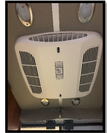
Picture 36.3 Roof-mount air conditioner
