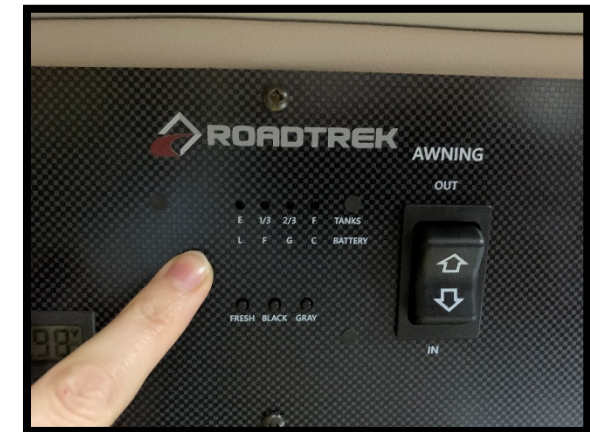
Picture 43.1 Tank Indicators
