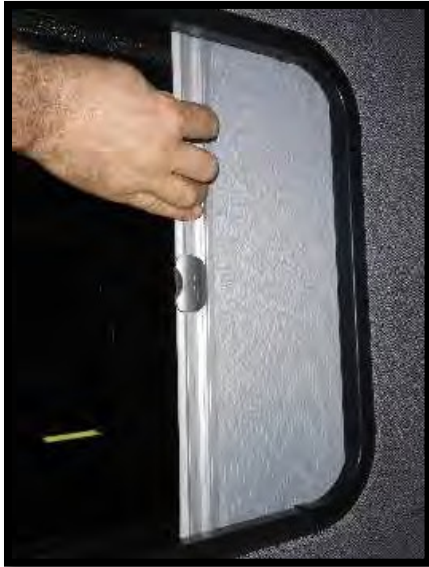
Picture 19.1 The side window screens – nightshade side
