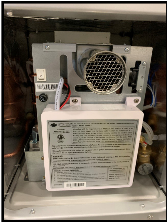
Picture 29.2 Girard water heater
