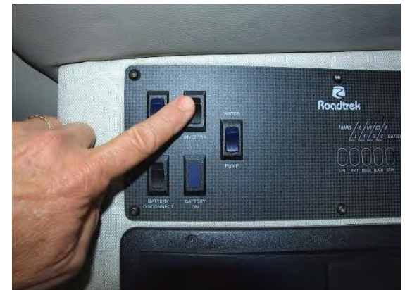
Picture 38.2 Inverter switch
