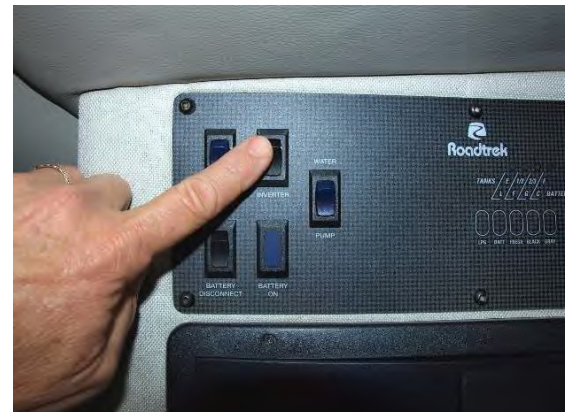
Picture 38.2 Inverter switch
