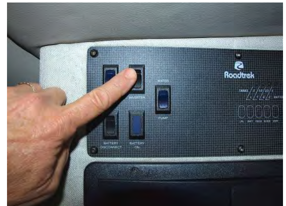
Picture 38.2 Inverter switch
