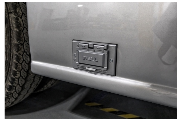
Figure 57.4 Prise extérieure 110 V.
