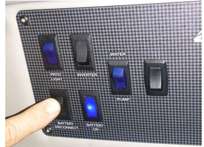
Battery disconnect switch
