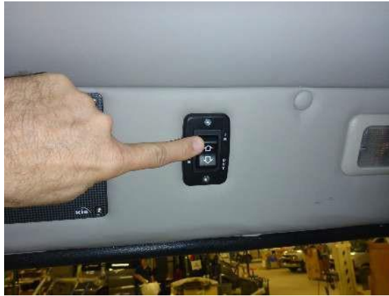
The awning power switch
