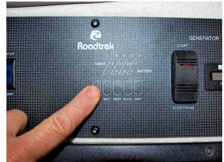
Tank level and battery charge indicators on monitor panel
