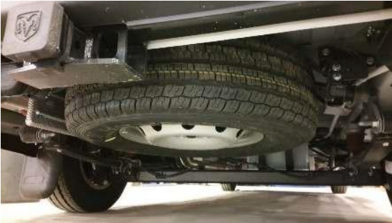
The spare tire is located is located behind the rear bumper
