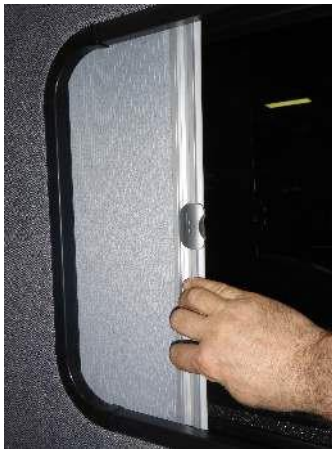
The side window screens – nightshade side
