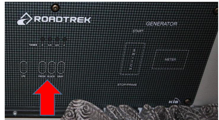
Tank level and battery charge indicators on monitor panel
