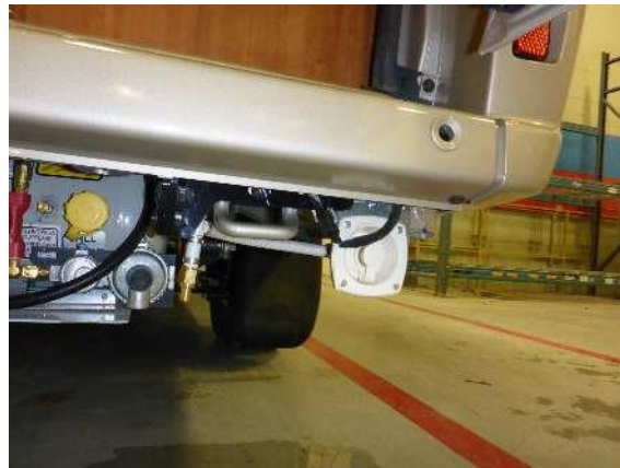
City water connection
