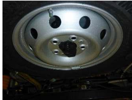
The spare is held in with a positive engagement spring.
