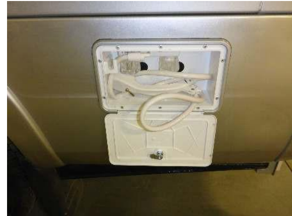
Rear compartment with outside shower faucet
