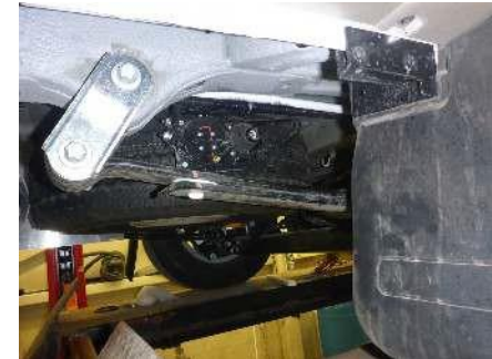
This lowering mechanism is behind the passenger side rear wheel
