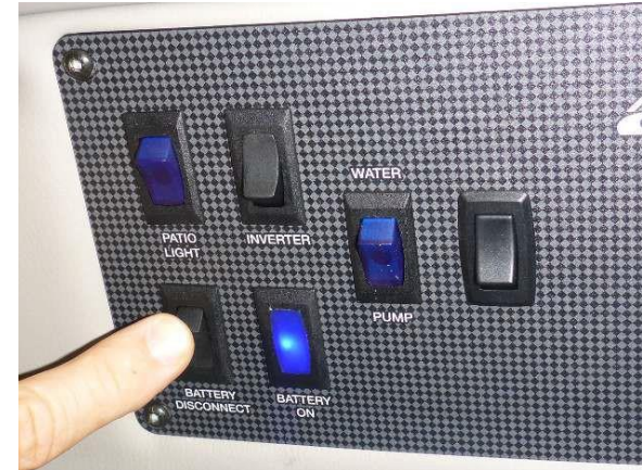
Battery disconnect switch
