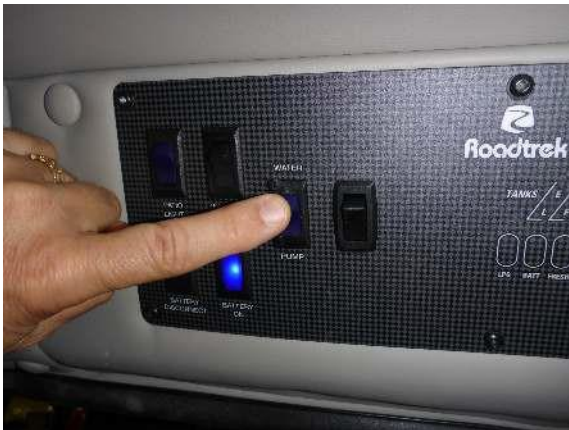
Water pump switch location on monitor panel
