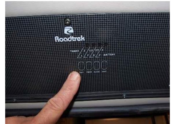
Tank and battery level indicators
