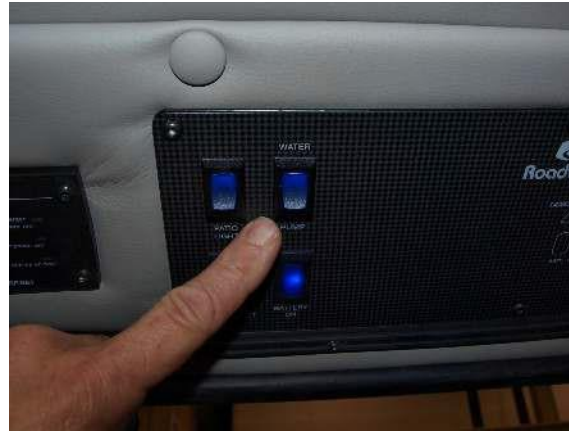
Water pump switch
