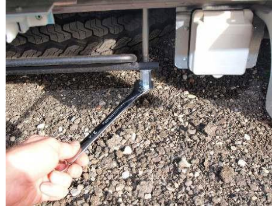
Use supplied wrench to loosen nuts 1/2 inch or so
