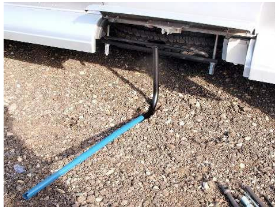
Lever in place to take the weight off the bolts
