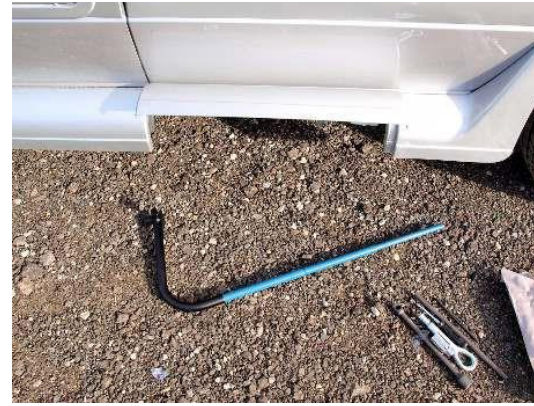
Assembled lever to lower spare tire carrier
