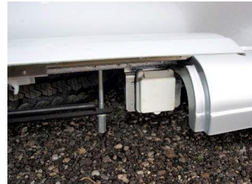
Shore Power connection point
