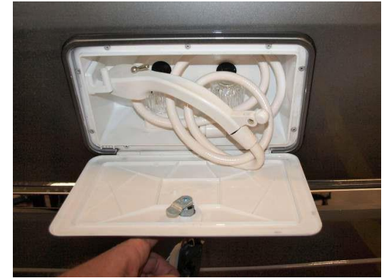
Outside shower compartment open, showing hose, faucet, and showerhead
