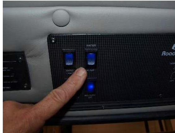
Water pump switch
