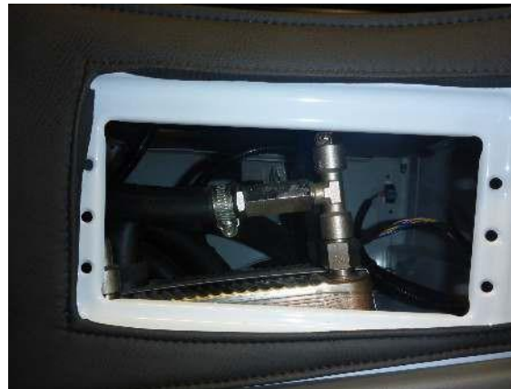
The heat exchanger valve open (as shown) allows the heat exchange to take place
