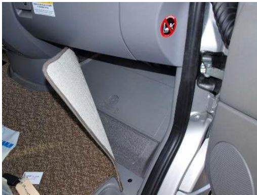
Tool access in front passenger footwell. Use a coin to turn the retaining clip and access the compartment.
