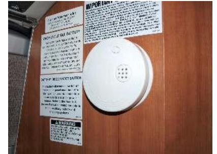
Propane and Carbon Monoxide alarm
