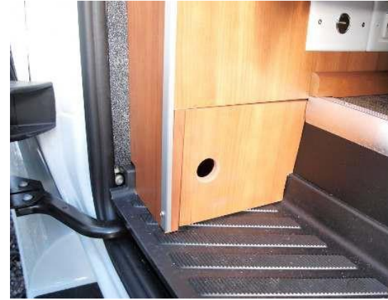
Valve access panel, on left end of side door opening
