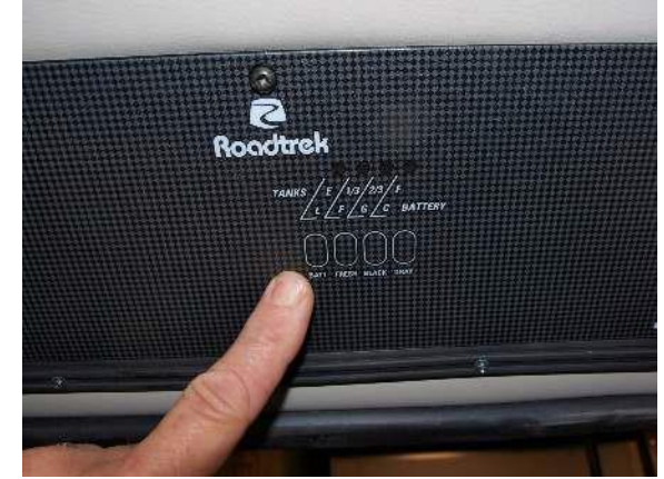
Tank and battery level indicators
