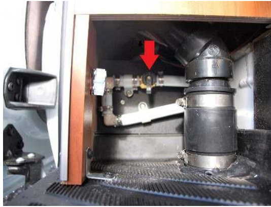
City water valve, shown closed (water is taken from on board tanks)
