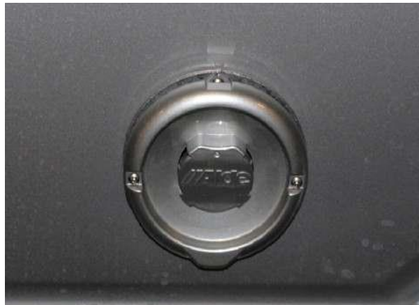
Vent for Alde unit on drivers side exterior
