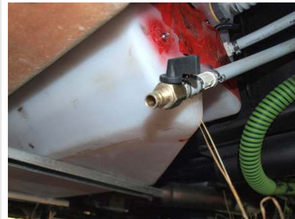
Exterior tank drain, located under the driver's door step. To open the valve and drain the tank, turn the handle so that it points along the water line.
