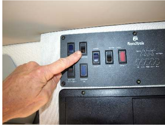
Inverter switch for standard 750 watt inverter
