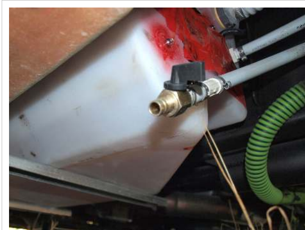
Exterior tank drain, under driver's door step
