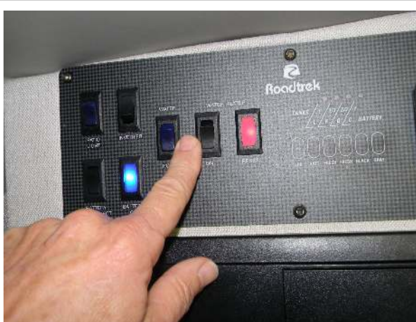
Water heater switch and red indicator light
