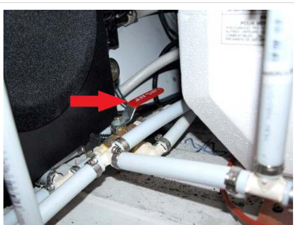
Tank selector valve in exterior tank position (colored plastic handle pointed toward driver's side of Roadtrek). This valve is located inside the hot water heater enclosure, just in front of the tank isolator valve.
