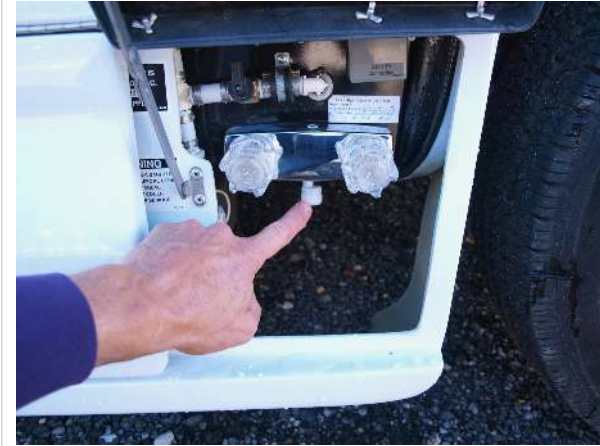
Driver's side rear access door, showing outside shower connection
