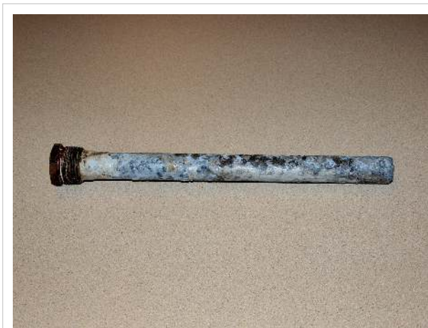
Water heater anode used up
