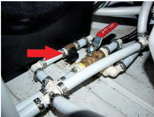
Location of the intertank valve shown in the open position
