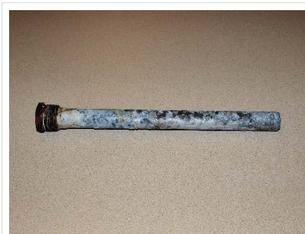
Water heater anode used up
