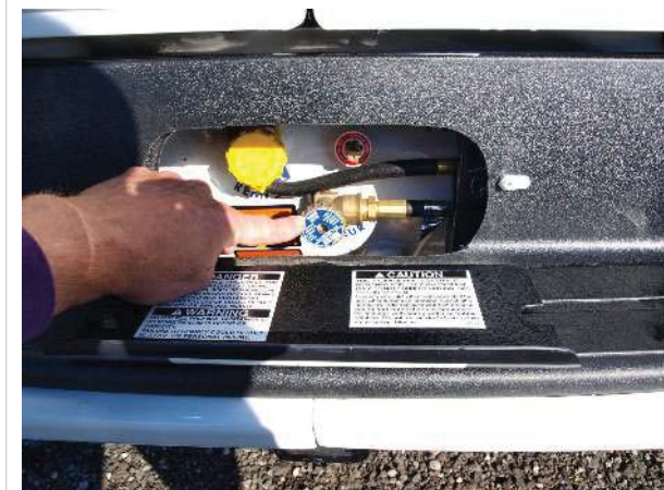
Propane tank main shutoff
