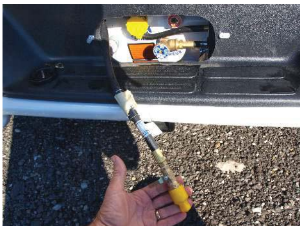
High pressure BBQ pigtail, shown with yellow dustcap and valve in closed position
