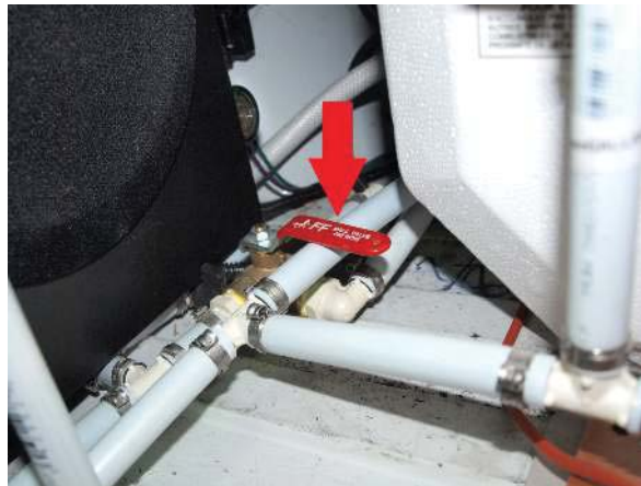
Tank selector valve in interior tank position, with the colored plastic handle pointed toward the front of the Roadtrek.
