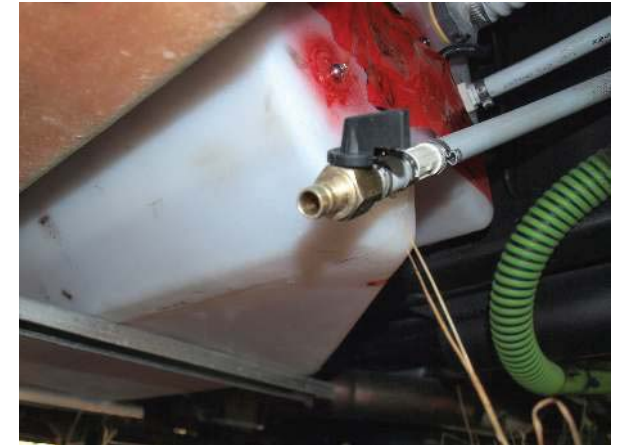
Exterior tank drain, located under the driver's door step.
