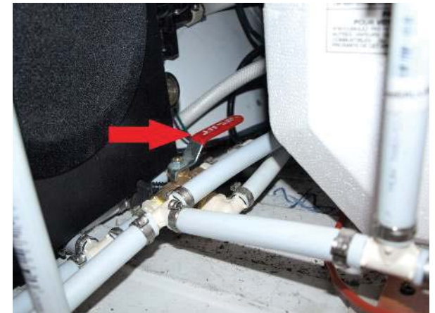
Tank selector valve in exterior tank position (colored plastic handle pointed toward driver's side of Roadtrek).
