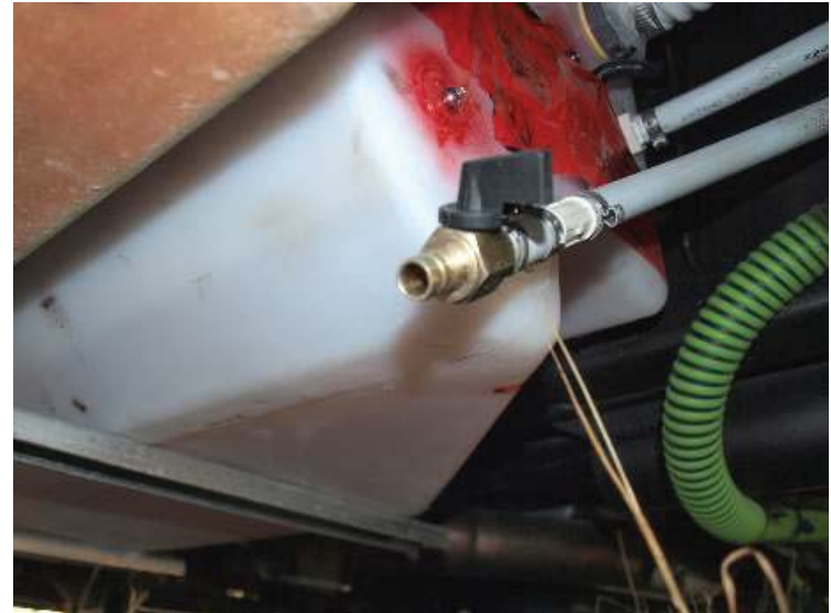
Exterior tank drain, under driver's door step
