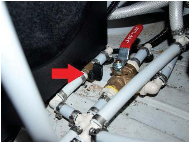
Valve connecting the interior and exterior tank, shown closed
