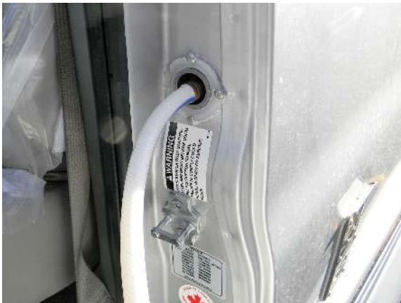
Filling the exterior tank
