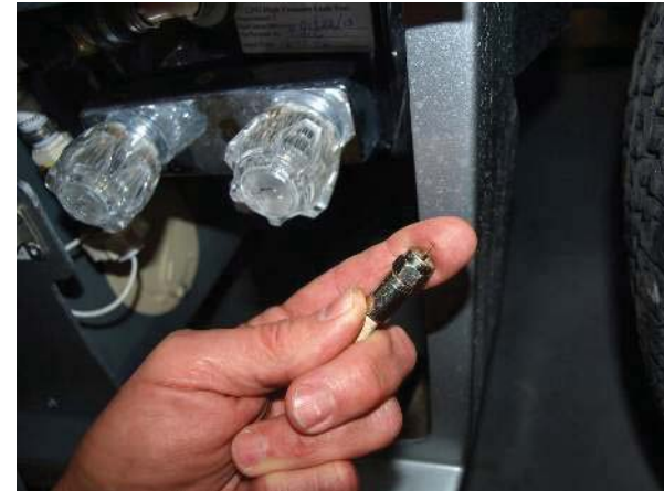
Coaxial TV connecting wire with screw-on end
