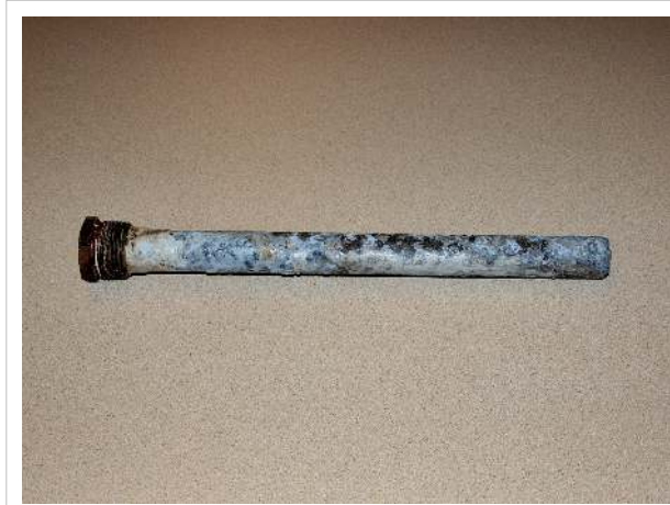
Water heater anode used up
