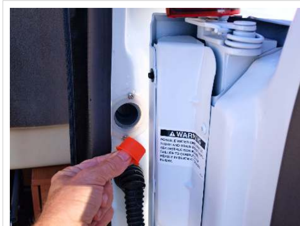
Rear (internal) tank gravity fill
