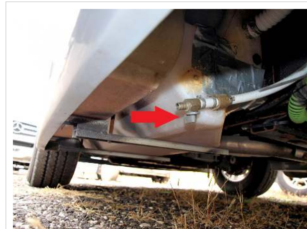
Fresh water tank drain, under driver's doorstep
