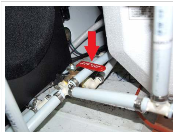
Tank selector valve in interior tank position, with the colored plastic handle pointed toward the front of the Roadtrek.
