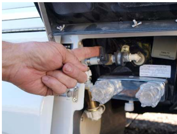
City water valve in closed (handle vertical) position
