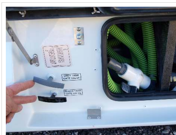
Waste water discharge hose with black and gray water valves
