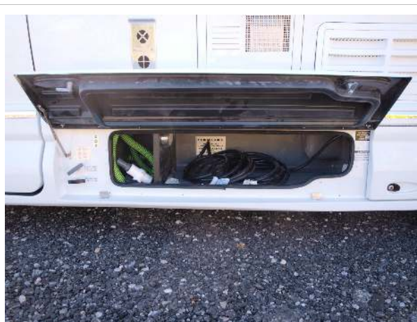
Compartment with waste water discharge hose
