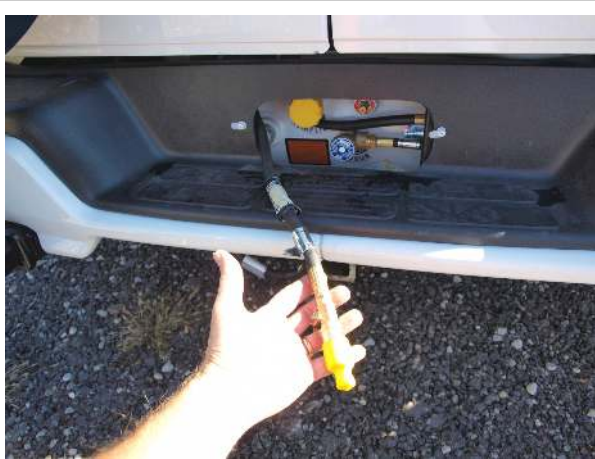
High pressure BBQ pigtail, shown with yellow dustcap and valve in closed position
