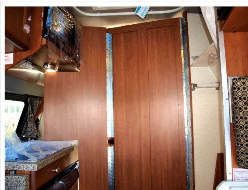
Door extended into privacy position
