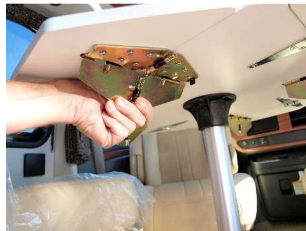
Fold the hinge flat to put the leaf back into storage position
